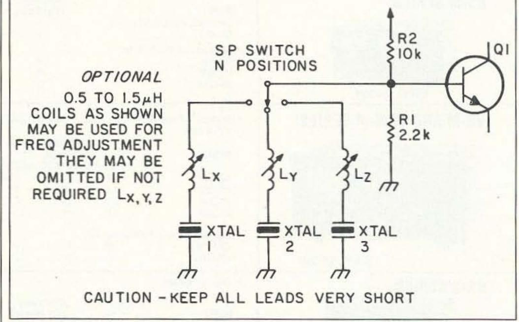
Figure 3. Scheme for XTAL switching.
